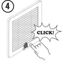
The front cover have to be unlocked through a lever lock (1) and swivelled upwards (2), the filter mat can be removed or replaced (3). If the front cover is closed again, you get an acoustic feedback by the engagement of the lever lock (4). The filter mat can be cleaned up to 10 times. In the standard version a filter mat of class G3 is used.
